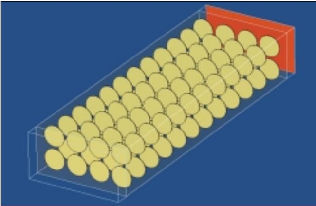
Figure 16: Layer arrangement of the 12 layer bandpass filter
