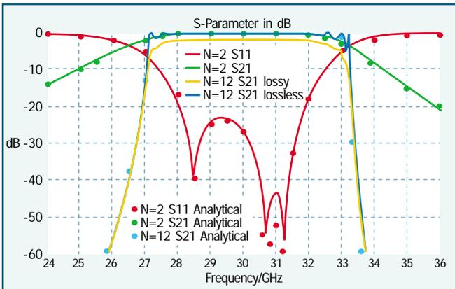
Figure 17: Passband filter characteristic for 2 and 12 layers
