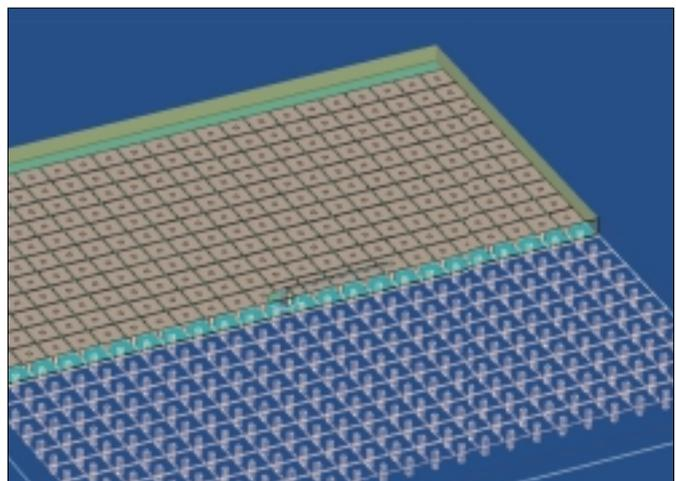
**Figure 5:** Wire antenna over a PBG structure
