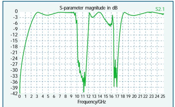
A coarse model applying default mesh-settings containing 43000 cells was simulated on a Pentium III, 800MHz, 512MB RAM, with a total CPU-time of 19 minute by applying online AR-filtering. The upper cut-off frequency was lower than the measured one by 3%, the lower one agreed very well with measurements.
