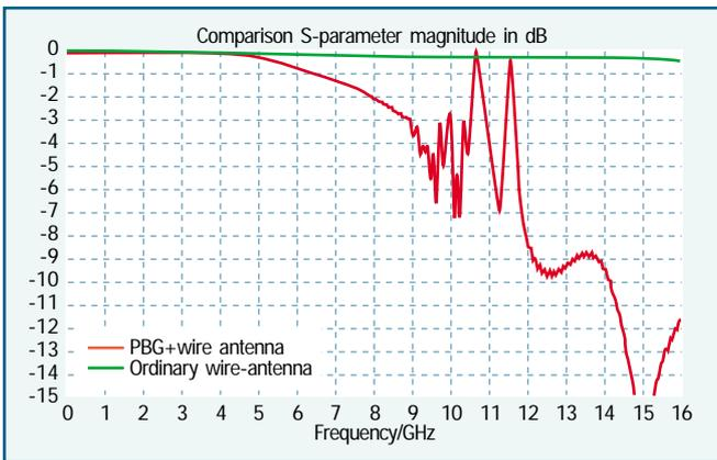
Figure 8 (left): Return loss of the horizontal antenna on two different ground planes
